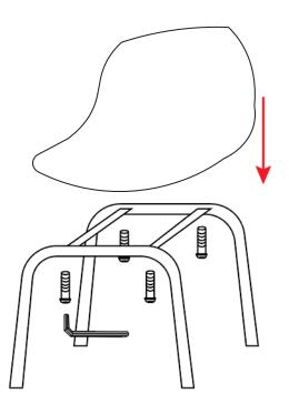
1. Insert four screws into the holes in the chair base. Using the Allen wrench, tighten them into the seat.
